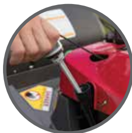
Automotive-Style Dipstick With Optimized Positioning
