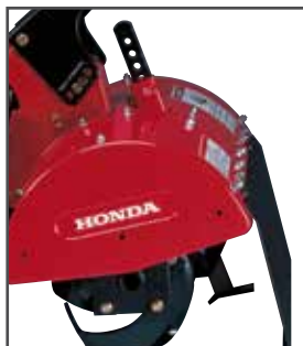
Adjustable Depth Bar This convenient feature lets you change the tilling depth.
